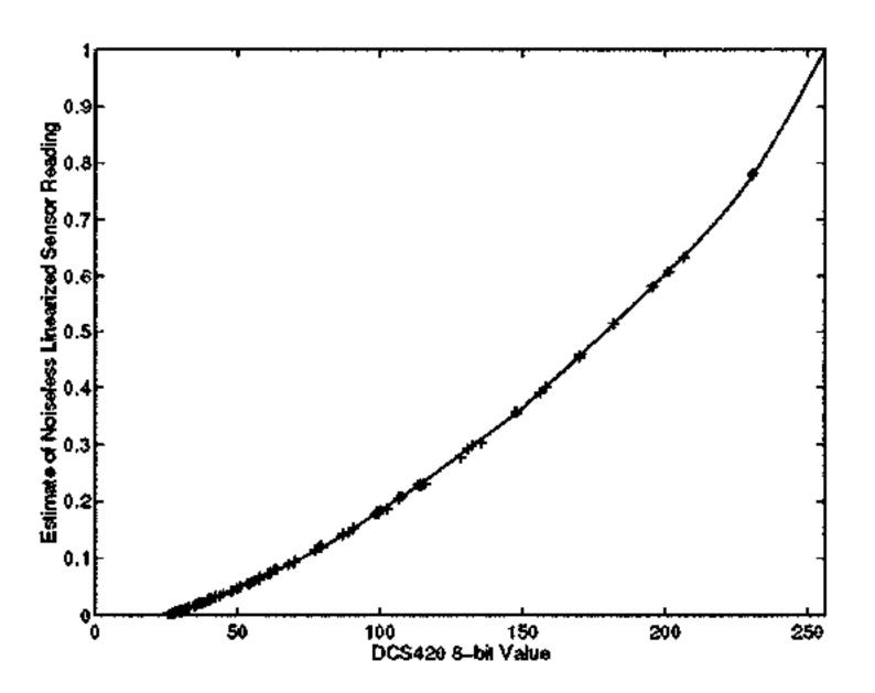
Figure 2: Calibration Curve - DCS-420.
