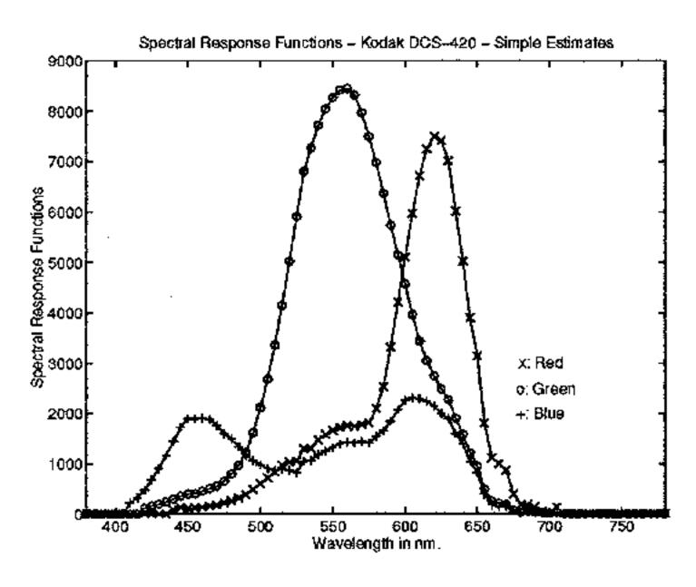
Figure 4: Spectral Response Functions of the Kodak DCS-420 - Simple Estimate.
