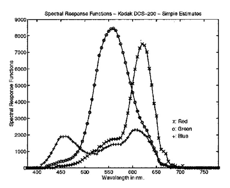
Figure 3: Spectral Response Functions of the Kodak DCS-200 - Simple Estimate.
